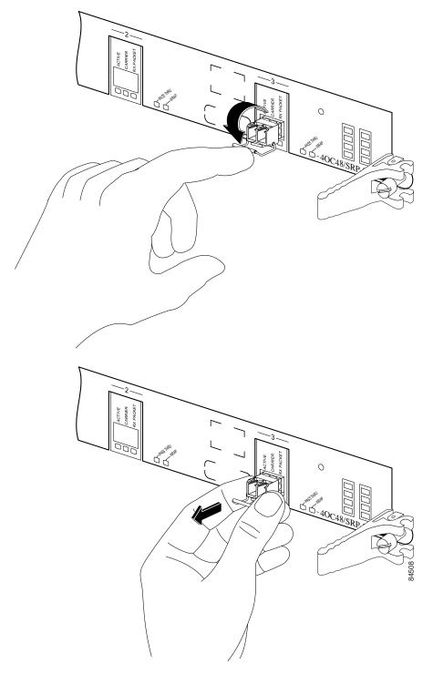
Figure 18 Removing a Bale Clasp SFP Module
